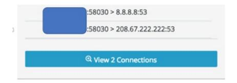
The screenshot below shows the traffic generated by the backdoor and demonstrates DNS Tunneling for C2 communication. As shown, while the destination IP is "8.8.8.8" – Google's DNS server – the malicious domain is "hiding" inside the DNS packet:
